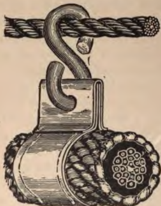
FIG. 254.—One form of cable hanger for suspending an aerial cable to the messenger wire.
